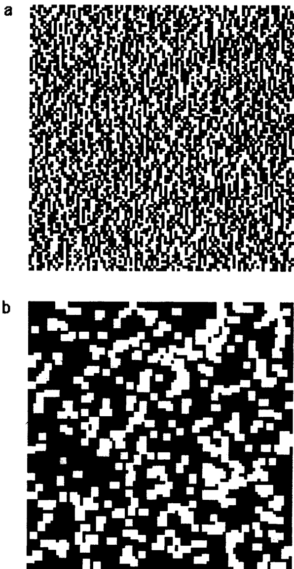
Figure 6. Simulated stereochemical structures (a) for the trans polymer and the corresponding crystalline regions (b) after annealing. See text.
