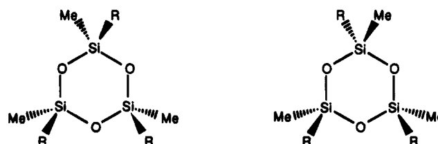
Figure 1. Sketches of the cyclic trimers, where R represents the (CH 2 ) 2 CF 3 group. The molecule to the left of the cis form, and that to the right is the trans form.
